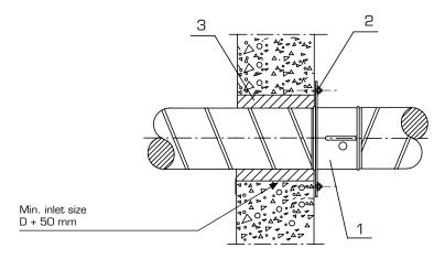
Installation of fire damper into building elements (walls and intermediate floors) made of concrete or masonry, construction thickness  $\geq$  110 mm. The blade shaft can be placed in any position.
