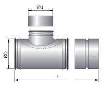
FWD length L (consists of pieces BDEG+BDEM+BDET) L = 200 mm Ø100 - Ø200, 310 mm Ø250 - Ø315 and 430 mm Ø400 - Ø630.
