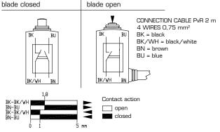
ELECTRICAL PROPERTIES: OPERATING TEMPERATURE -25 ... +70°C AC-15: B300 (Ue=230VAC, Ie=1,5A) DC-13: R300 (Ue=24VDC, Ie =3A)
