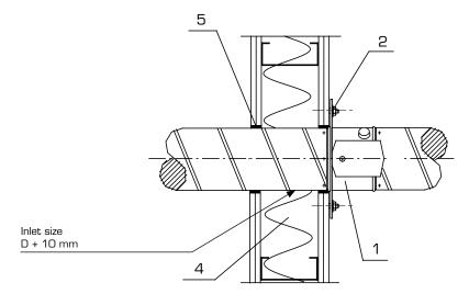
Installation of fire damper into lightweight plasterboard building elements (gypsum board or similar), wall thickness ≥ 116 mm. The blade shaft can be placed in any position.
