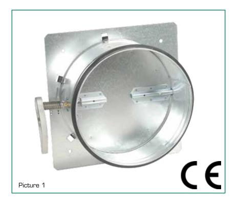
Fire and smoke damper ETPR-E-1 is used as a closing device for preventing the spread of fire and smoke in ventilation ducts between fire compartments. Fire dampers are equipped with fusible link and spring mechanism for closing (see picture 1) or with electrical actuator (see picture 2).
